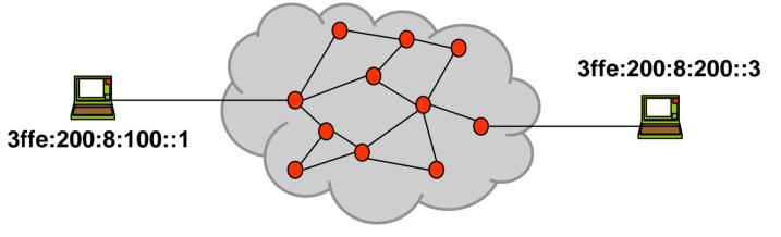
Connection = {source IP, source port, dest. IP, dest. port}
