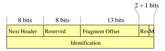
Next Header<br/>part of theIdentifies the initial header type of the fragmentable<br/>original packet.Fragment OffsetThe offset of the data following this header.M flag<br/>Identification1 = more fragments; 0 = last fragment<br/>Unique identifier for each fragmented packet.
